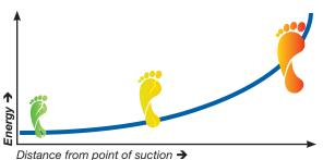
Distance from point of suction → The graph demonstrates the relationship between environmental impact and the distance of the pump from the point of suction.
