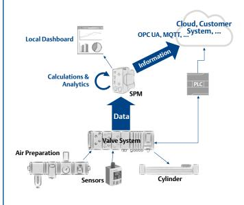
Want to check the state of wear? Need information on energy efficiency? The new Smart Pneumatics Monitor will provide you with reliable answers. It sends status messages to defined employees and parent IT systems without detouring via the machine controller. This minimizes the risk of machine downtime and substantially lowers operating costs.
